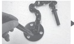
Insert the anchor bolts with nut attached into the holes through the floor plate. Using the 13 mm spanner, progressively tighten down each of these anchor nuts so that all three bolts are firmly anchored into the concrete.
