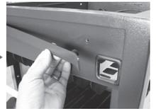
Slide the sleeve on the rear of the Weather Cover bag over the cleat.
