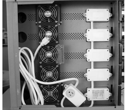
If no pedestal is being used under the stack, plug the top FUYL Cell into the 'hidden' socket - located inside the left cover of the FUYL Cell below.
